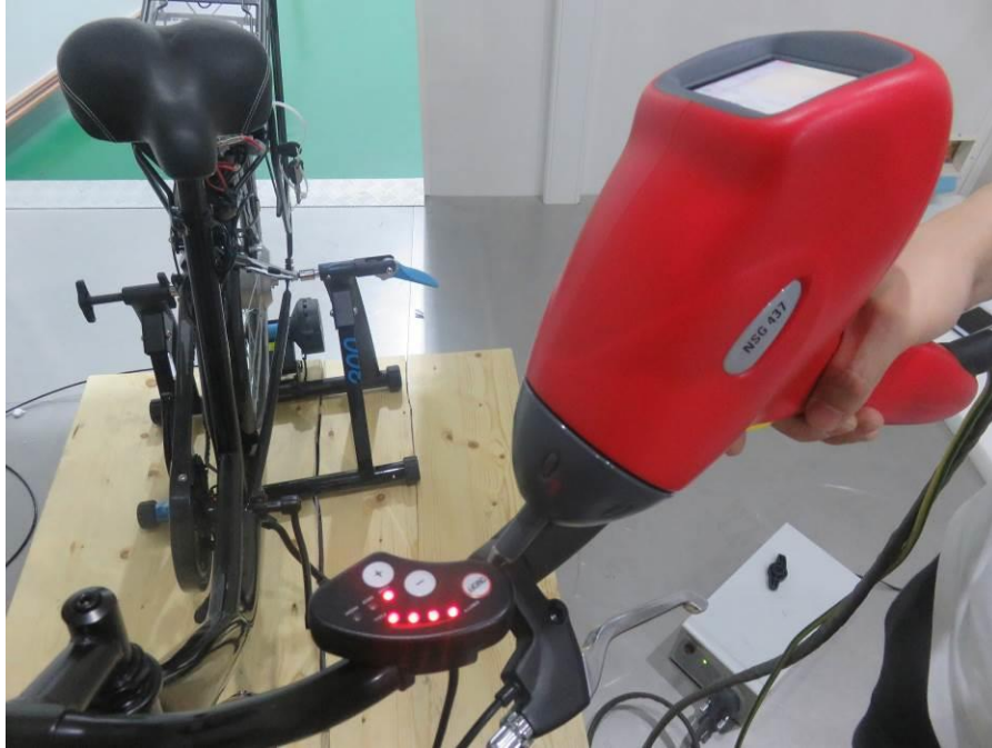
Photograph 3: Set-up for ESD immunity test
